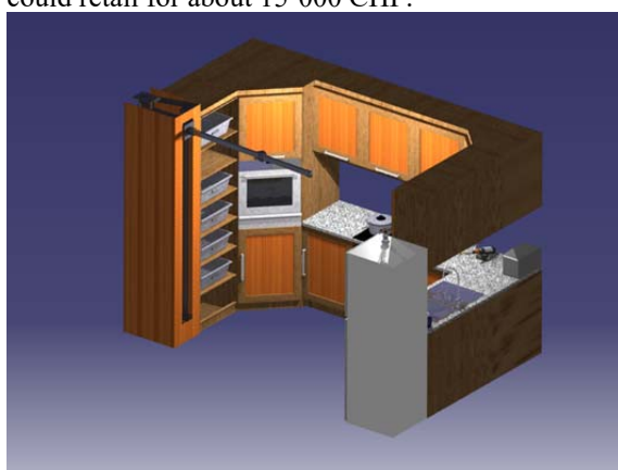
Figure 4: Simulation of an assistive kitchen arm (far left). The arm moves up and down and can place/extract trays from the shelving beside it onto the work surface as well as move objects in and out of the oven.
