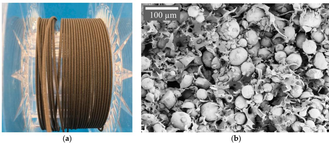
**Figure 2.** (a) Polymer-bonded magnetic filament flexible enough to be spooled on a standard filament spool with a diameter of 10 cm; (b) SEM micrograph of the extruded polymer-bonded magnetic compound, NdFeB particles inside the POM/PA12 matrix.
