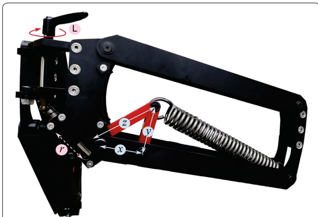
Fig. 9 Image of the prototype. The lengths x , y and z are highlighted. By rotating lever L the lower end of beam z can be positioned along the range r to adjust for different external loads F_z
