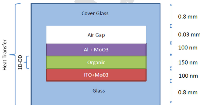
FIG. 1. Structure of HOD and thickness of layers. The heat equations are solved on the entire device domain, while the drift-diffusion model is only solved in the organic layer.
