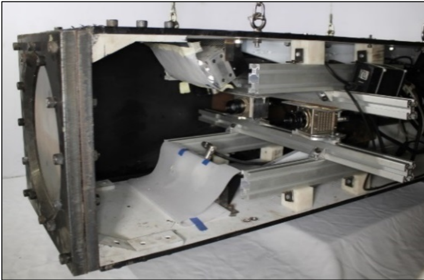
Fig. 4- Photograph showing the inside of the modified pendulum, set up for filming the rear surface of the plates
