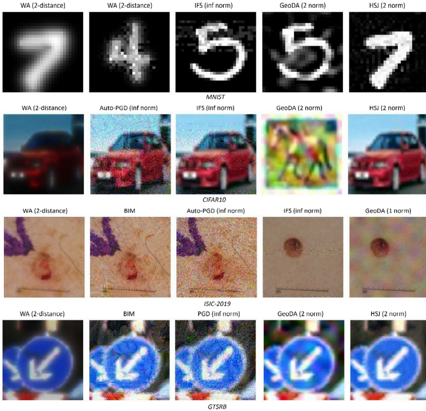
Fig. 4. Generated adversarials with different patterns depending on the attack and the utilized norm or p -distance used. Adversarials generated with the first or second norm or p -distance tend to create patterns with a small subset of adversarial pixels, while adversarials generated with the inf norm tend to create a broad adversarial pattern across the whole image.
