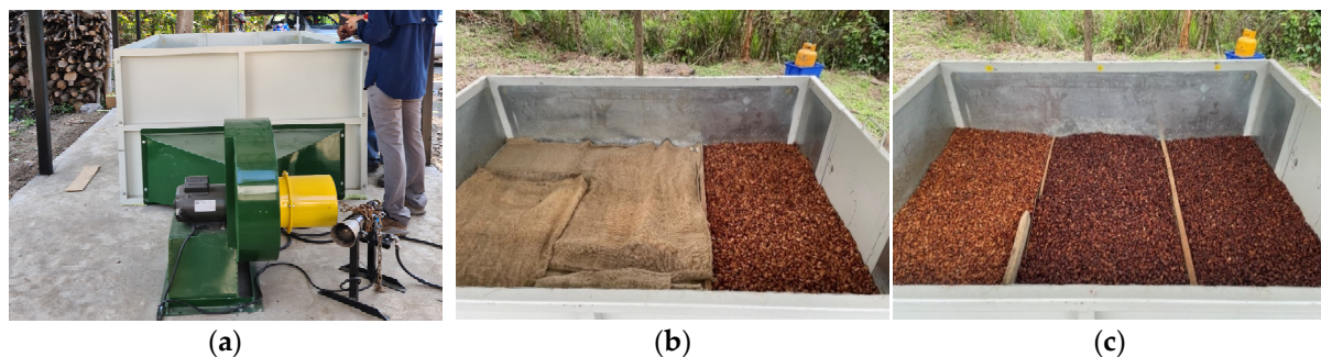
Figure 3. (a) Artificial dryer SIRCA (Model: SR-10-SI) at location F; (b) beans from variation PS0_H in 1/3 of dryer and rest covered with jute bags at location A; (c) beans of variations PS5_L, PS3_L, PS0_L separated in dryer with wooden sticks at location A.
