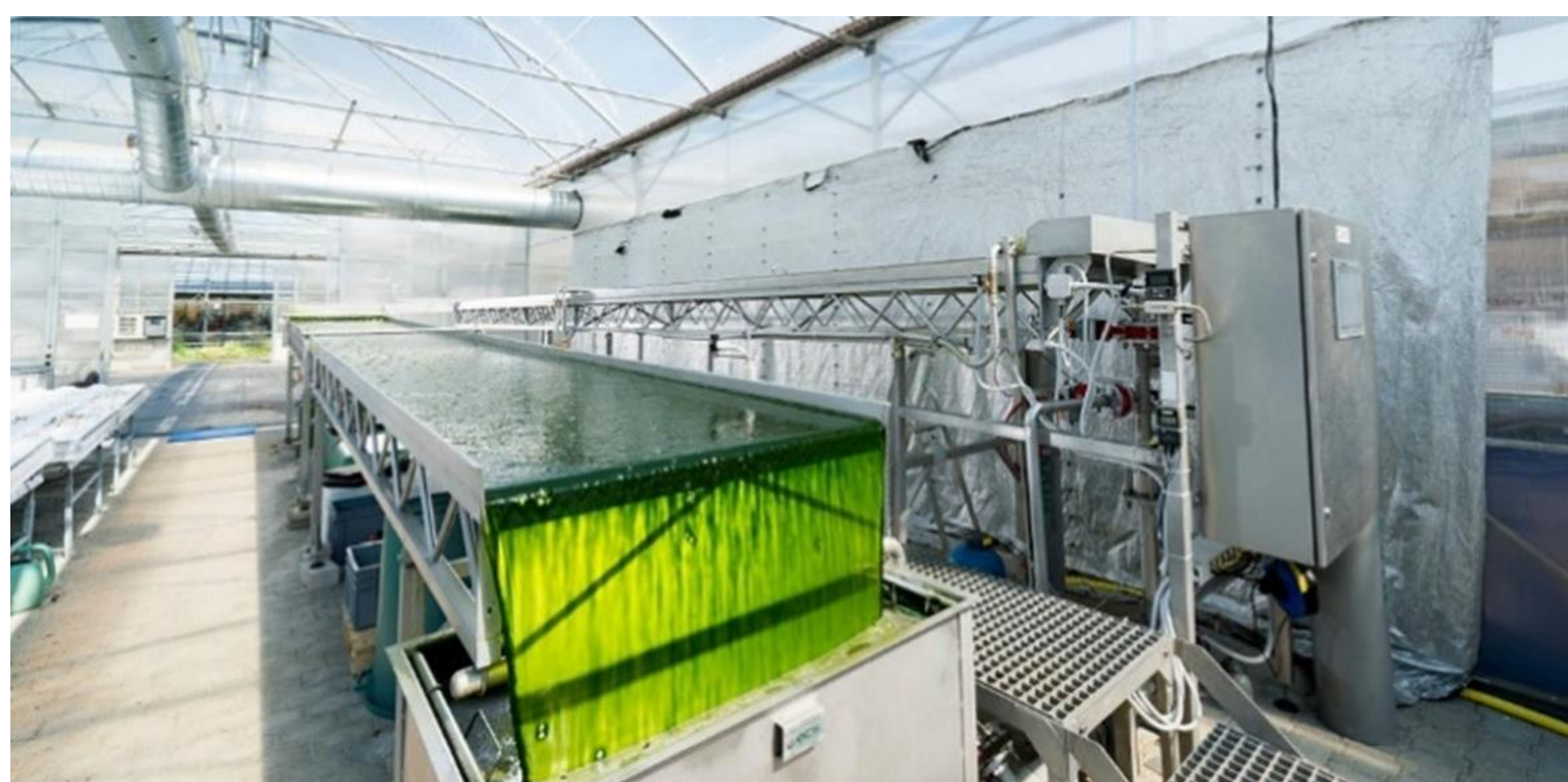
Figure 1. Thin-layer PBR for cyanobacteria production, located at the Institute of Natural Resource Sciences of the Zurich University of Applied Science. Photo: Frank Brüderli
