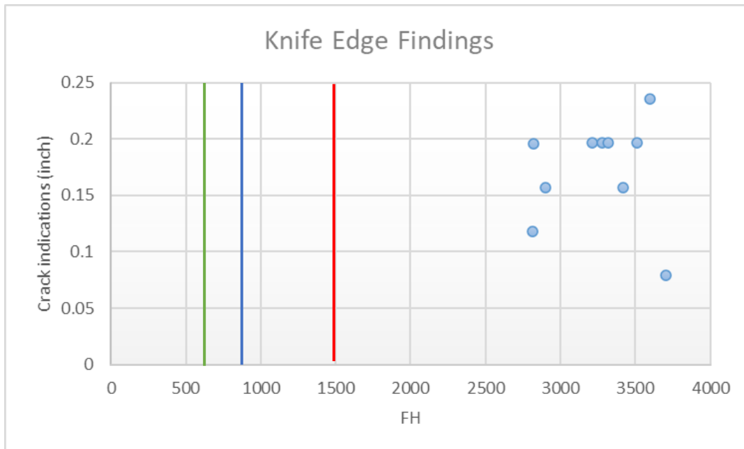
Figure 8: Knife Edge Fleet findings. The red vertical line is the threshold to 1e^{-5} from the Freudenthal calculations. The green and blue line are the same thresholds from Lincoln (SMART|DT and PROF3.2).
