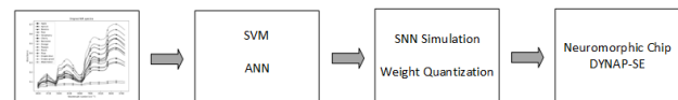
Figure 1: Pipeline overview. We used the NIR-spectral data as direct input for the neural networks. We started with building SVMs as a reference, then built an ANN, which was converted into an SNN and simulated with quantization-aware training. Finally, the chosen architecture with trained weights was transferred onto the neuromorphic chip DYNAP-SE.
