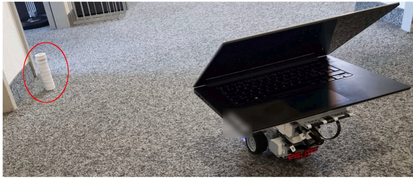
Fig. 8. Robot driving to the circled beacon stack destination. The laptop acts as bluetooth receiver and edge voter.
