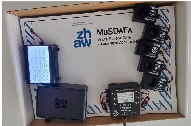
Fig. 6. Portable 'shoe-box' testbed for our light sensor setup (Fig. 5). A Raspberry Pi 4 runs the fusion script. An LCD display shows the voting results and weight values.
