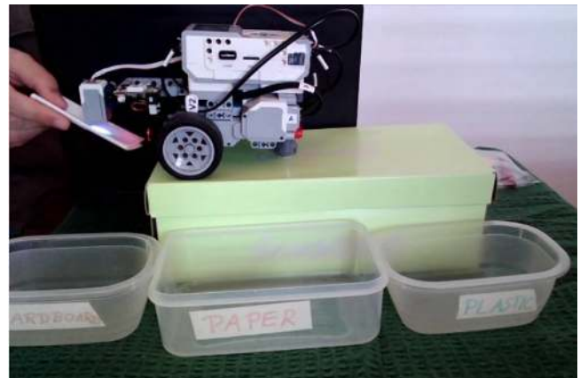
Figure 5: Exemplary teaching setup of the 'interactive smart bin' scenario with only the two colour sensors in operation
