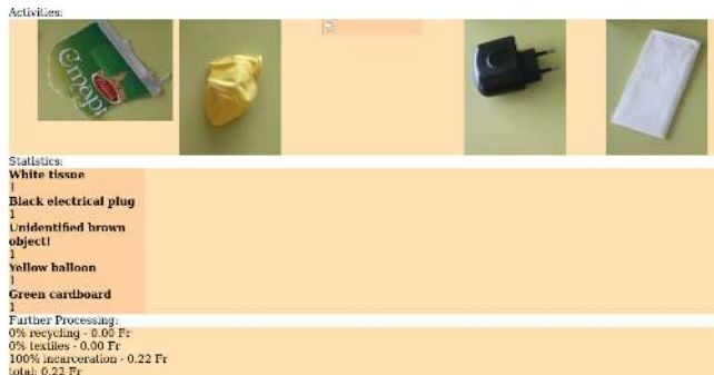
Figure 3: Information screen for disposal system operators
