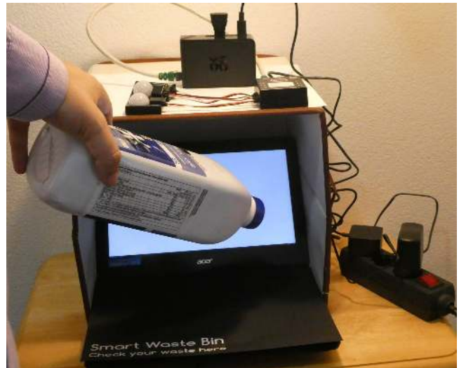
Figure 4: Recycling station setup of the 'interactive smart bin' scenario
