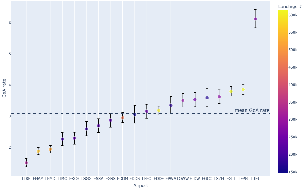
Figure 3. Observed GoA rate per airport type and the 95% CI. The dashed line refers to the mean GoA rate per airport.
