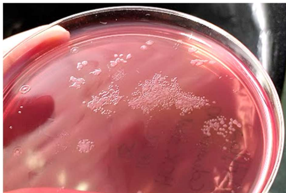
Figure 17: Outflow column 10 (Sand supplemented with HCK), before E. coli flushing. The grown colonies on the agar plate must originate in the column.
