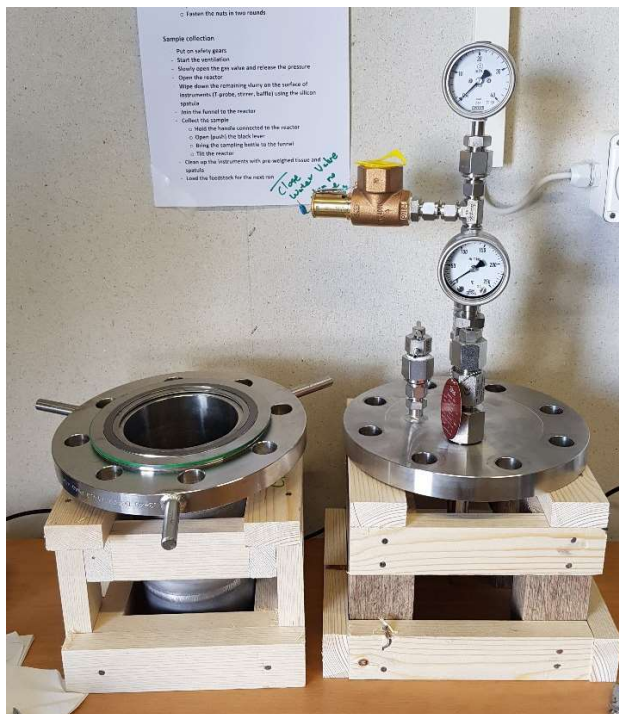
Figure 3: BLR reactor (left) and lid (right) with temperature and pressure sensor as well as pressure emergency release vent.
