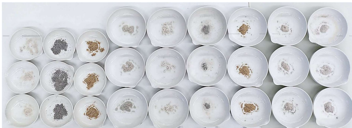
Figure 13: Ash colour of the different materials. CG, KW, GW, TW, HCC, HCK, HCG, HC200, HC180 (from left)
