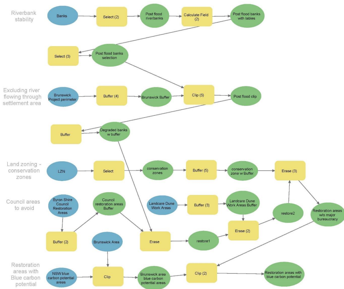
Figure 4: ArcGIS ModelBuilder for finding potential restoration sites on the Brunswick River NSW. Two main outputs are given as a result: restoration areas without major bureaucracy areas, and with blue carbon potential.
