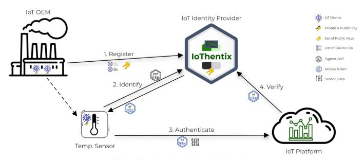
Figure 1: Overview token-based authentication flow
