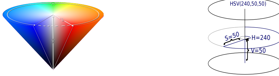
Fig. 3. HSV color model: On the left, the cone of possible colors for various hue color angles H , saturations S , and darkness values V are shown. H can take values between 0^\circ and 360^\circ , S and V between 0 and 100. The example of how to compose the color “navyblue” in this HSV color model is presented on the right. (pictures taken from wikipedia [28])
