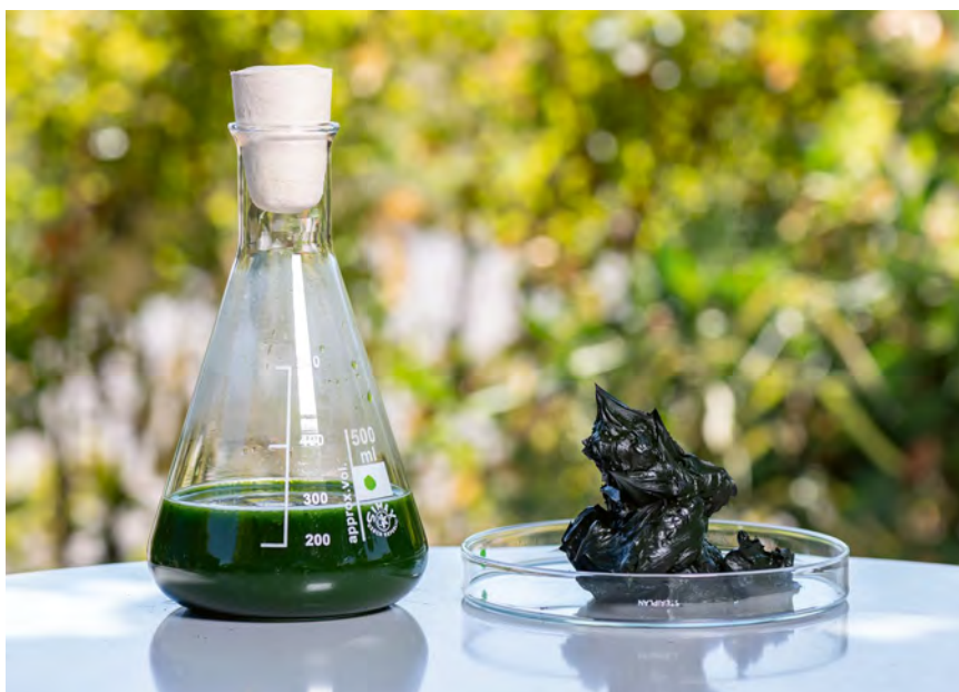
Fig.: Microalgae, as liquid culture (left) and as paste after dewatering (right). (photo: Tevy, Wädenswil)
