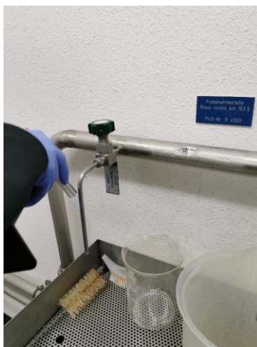
Figure 2: Sampling site for raw water with a tap at IWB Basel. (Source: Erb Severin)
