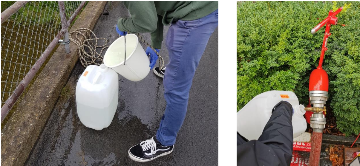
Figure 16: From left to right; Water sampling for raw water out of the river Thur; End of pipe sampling from a water hydrant in Bischofszell. (Source: Erb Severin)
