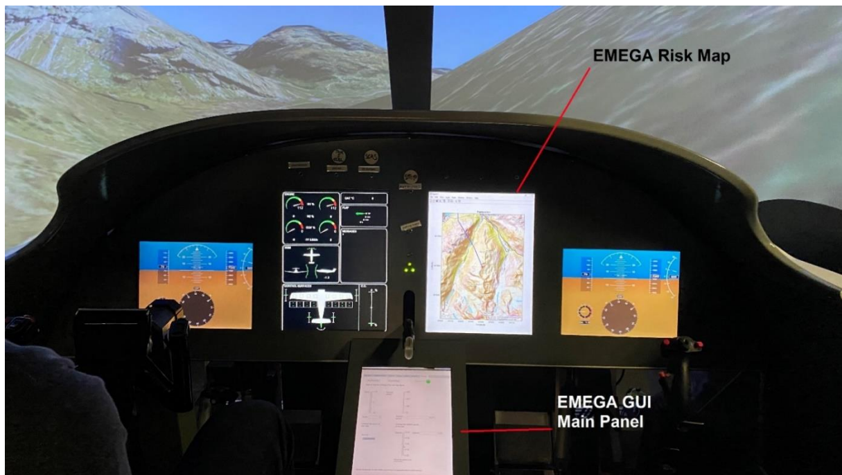
Figure 3 – EMEGA GUI integrated in the cockpit of the ReDSim
