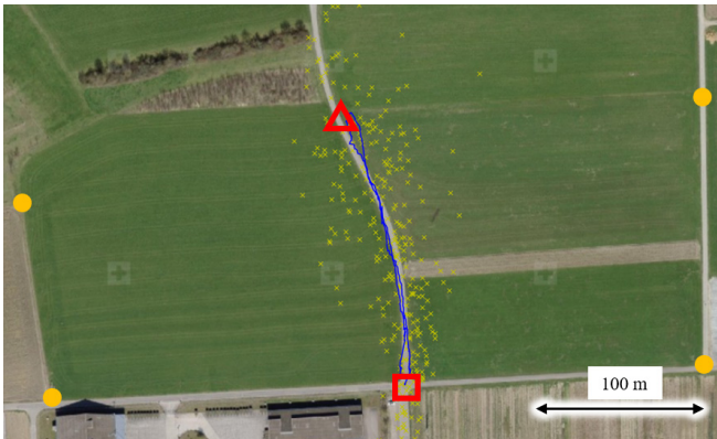
Fig. 7. Positioning Test with estimated positions using LoRa ranging directly (yellow crosses) and tracking with Kalman filtering (blue line). The orange circles indicate the reference nodes. Aerial view: swisstopo
