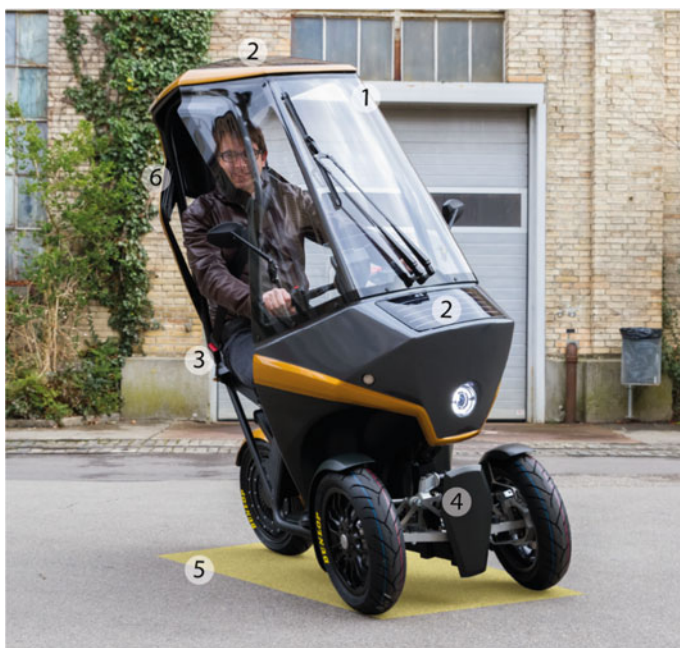
Fig. 1 BICAR—Main features: 1. weather protection incl. wiper system; 2. solar powered; 3. safety belt system; 4. three-wheel-tilting chassis; 5. needs only 1.2 m 2 parking space; 6. robust tubular frame
