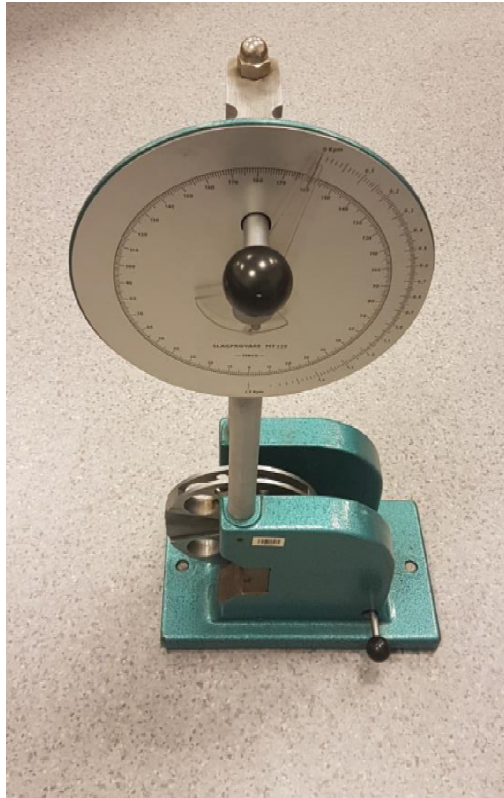
Figure 6: The Charpy testing machine used in this research.
