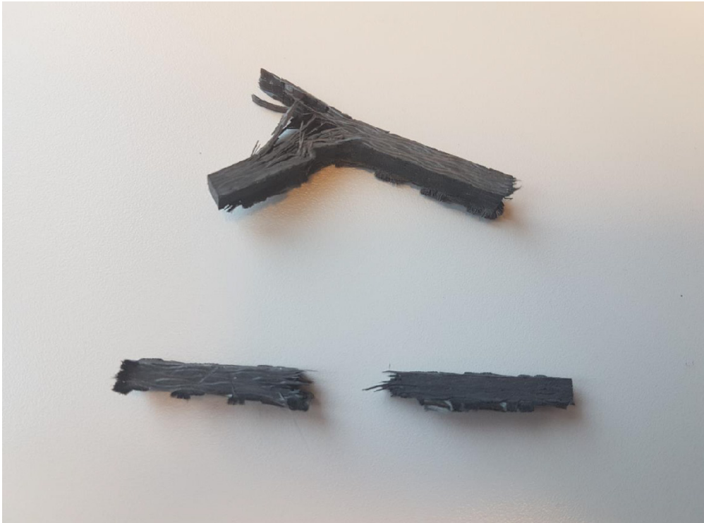
Figure 10: A visual display of the CFRP failure after Charpy experimental test.
