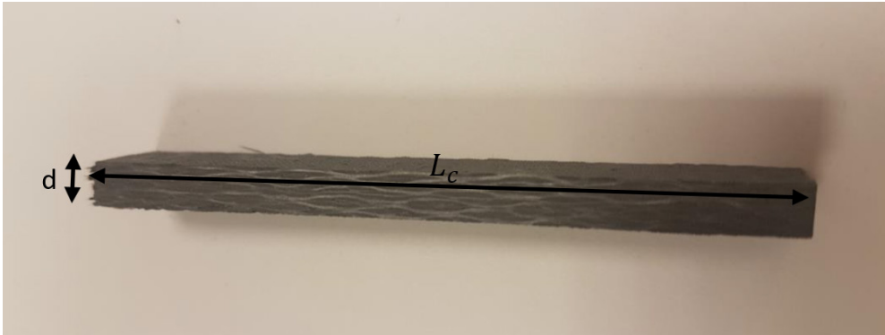
Figure 5: The span-to-thickness ratio ( L_c/d ) of a test piece of CFRP
