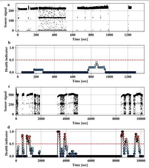
**Fig. 9** Fault detection using statistical analysis. **a** Sensor signal of healthy machine. **b** Health indicator for healthy machine. **c** Sensor signal for faulty machine. **d** Health indicator for faulty machine. Red dashed line indicates the detection threshold
