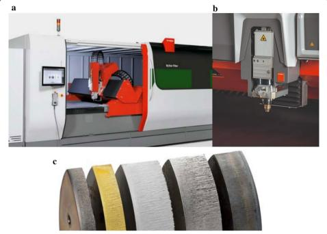
**Fig. 1** Intelligent maintenance: **a** A laser cutting machine, **b** the cutting process and **c** examples of materials and thickness
