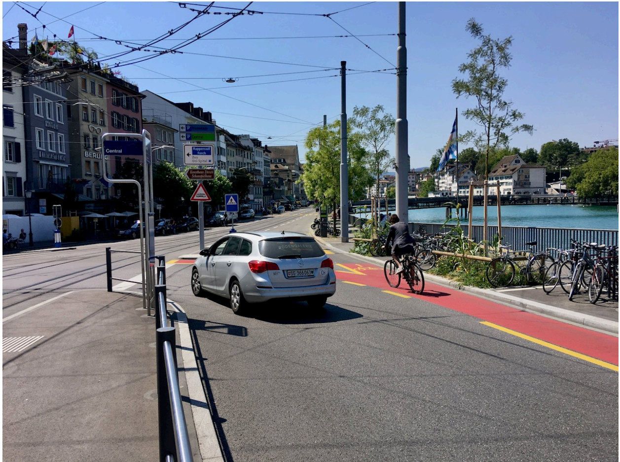
Fig. 1: Public transport lane, motor vehicle lane, bike lane and pedestrian promenade at Central-Platz Zurich, looking towards the Limmatquai. (Photo source: Andrew Nash)
