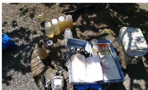
Figure 16 On-site measurement with the Multi meter HQ40 Source: Pravin G. Moorthy
