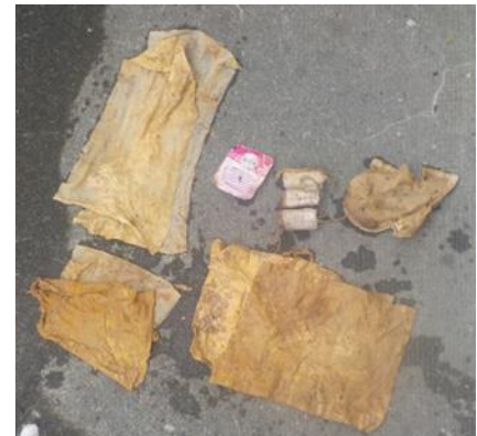
Figure 14 Waste products fished out of the first chamber of the septic tank Source: Autark Engineering
