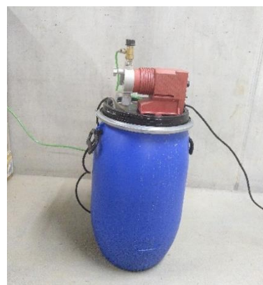
Figure 20 30L Container with peristaltic pump for activation and dosing Bioclean TM Source: Pravin G. Moorthy
