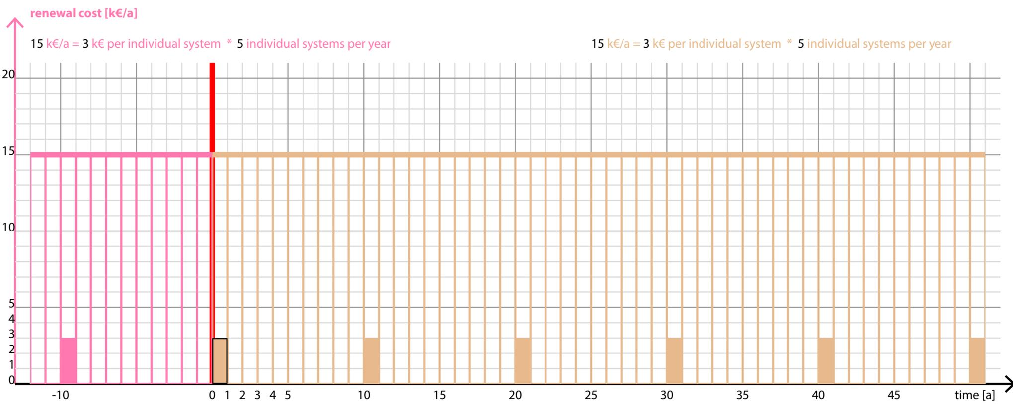
**A -> B, optimised running costs (- 33 %) after installing optimised systems within ordinary replacement cycle**
