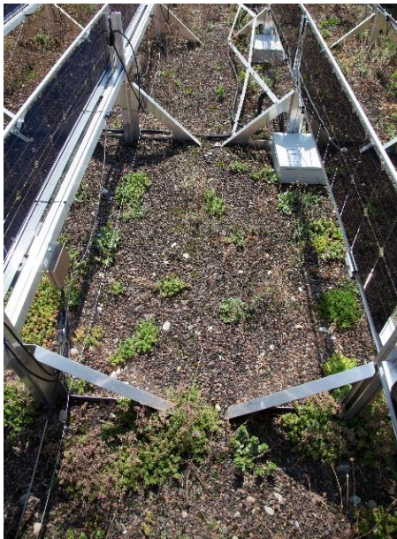
Figure 3 Photos of the two green roof areas that were measured with increased precision. On the left side is the standard green-leaved green roof (SGR) and on the right side is the “bright” silvered-leaved green roof (BGR). The photos were taken after a long dry and hot period on 21 st August 2018. The depictions demonstrate the higher resilience of the silver-leaved plants compared to the standard greening.
