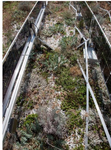
Figure 3 Photos of the two green roof areas that were measured with increased precision. On the left side is the standard green-leaved green roof (SGR) and on the right side is the “bright” silvered-leaved green roof (BGR). The photos were taken after a long dry and hot period on 21 st August 2018. The depictions demonstrate the higher resilience of the silver-leaved plants compared to the standard greening.
