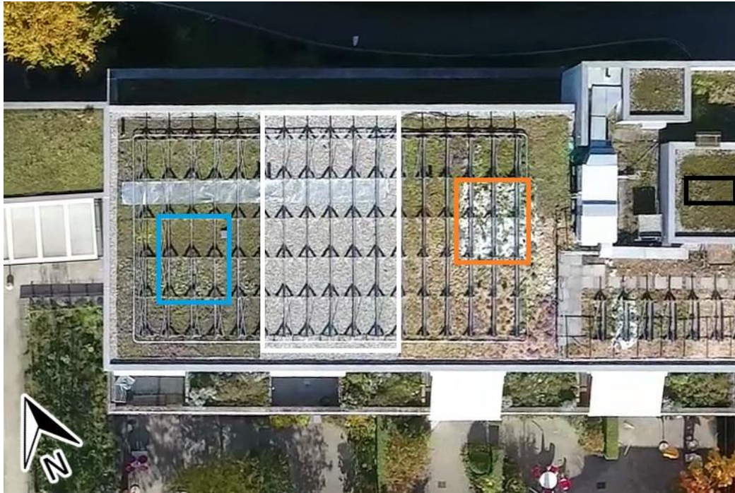
Figure 2 Aerial view of the roof. Power measurements with increased precision were performed on respectively two modules in the center of fields marked with orange and blue color rectangles. The monofacial south-oriented reference module (not shown on the photo) is located in the area marked with the black rectangle. The ground in the area within the white rectangle is covered with gravel. Due to the building orientation the alignment of the system is, compared to a perfect east-west orientation, rotated by 25°.
