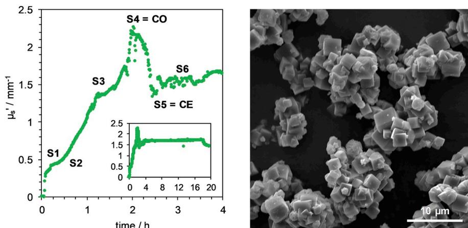
**Fig. 2.** Left: Reduced scattering coefficient  $\mu_s'$  at 636 nm during the first 4 h of the zeolite A synthesis (inset: entire duration). Samples were taken after 0.25 h (S1), 0.75 h (S2), 1.25 h (S3), 2 h (S4), 2.67 h (S5), and 3.08 h (S6), with S4 approximately representing the crystallization onset (CO) and S5 the crystallization end (CE). Right: SEM image of the final product obtained after 20 h of synthesis time.
