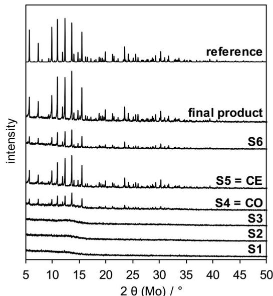
Fig. 4. Powder XRD patterns of in-process samples S1 to S6 and of the final product. The patterns are offset for clarity. A reference pattern for hydrated zeolite A [48] is shown for comparison.
