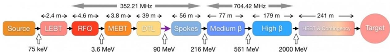
Figure 1: The ESS linac with its different sections, including lengths and nominal beam energies. Source: [esss.se/accelerator](http://esss.se/accelerator).
