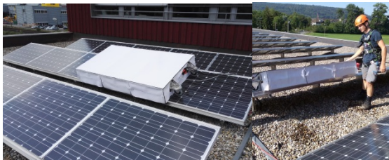
Figure 5: The PLF during the outdoor measurements at the PV Plant "Die Werke, Wallisellen".
