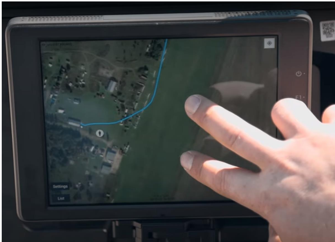
Figure 2: Screen of the portable version of AeroScope displaying a drone flight path [13]
