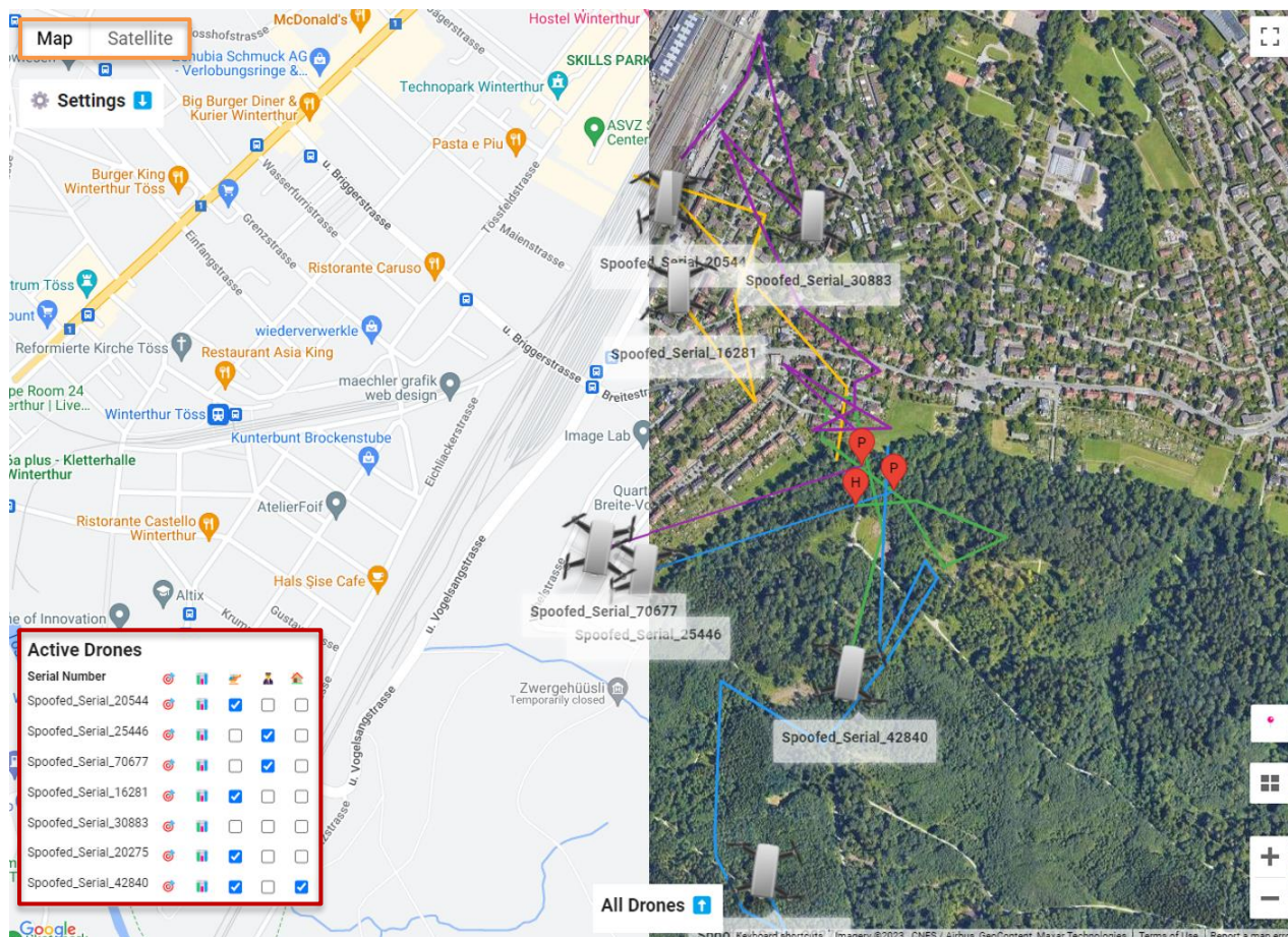
Figure 17: Monitor view with satellite map and the highlighted control elements
