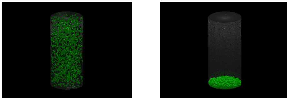
Fig. 1. Initial (left) and final (right) configuration generated in a simulation of the agglomeration process of a multidisperse system of 2,000 spherical particles in a cylinder.
